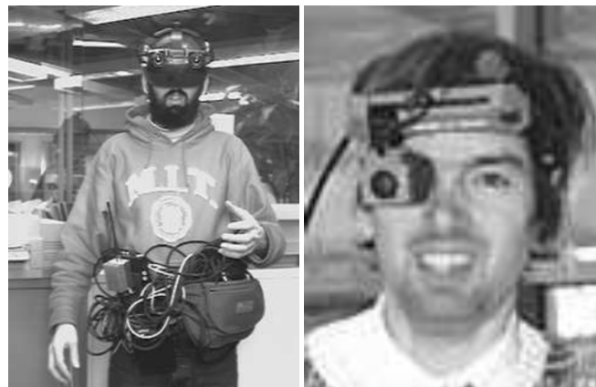
Figure I-41. Head Mounted Displays for mediated reality. (Left) A double-eyes visor. (Right) Single-eye visor example.
