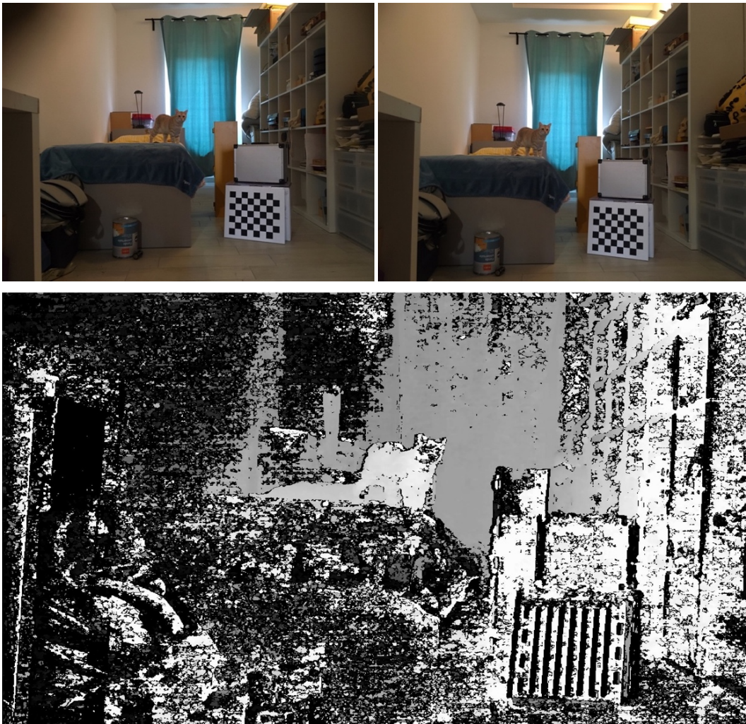
Figure I-38. Two photos taken with two smartphones with a horizontal displacement of a few centimeters and the corresponding disparity map obtained with MATLAB. In this image, lighter objects correspond to smaller distances from the camera.
