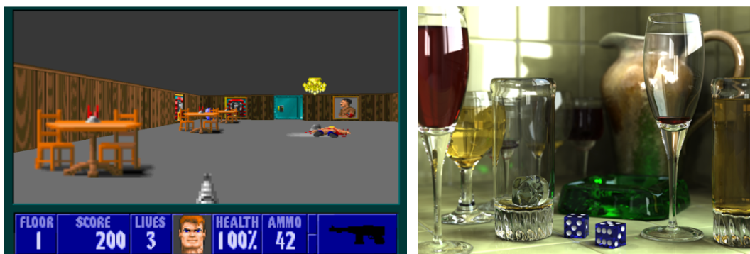
Figure I-9. (Left) Ray casting in a recent version of the classic Wolfenstein video game [153]. (Right) Result of a recursive algorithm in which each ray refracts and reflects multiple times. Caustic phenomenon can also be noticed. Camera effects such as depth of field and aperture shape are also here simulated.
