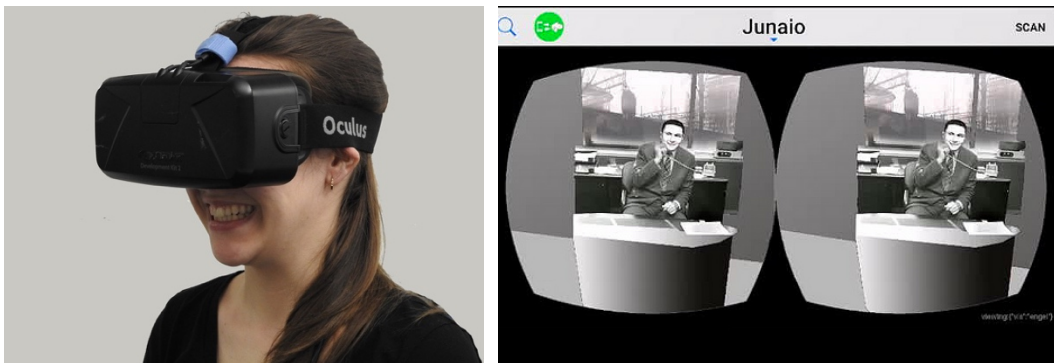
Figure I-55. (Left) The Oculus Rift device. (Right) An example of a stereo image that can be seen inside a HMD.
