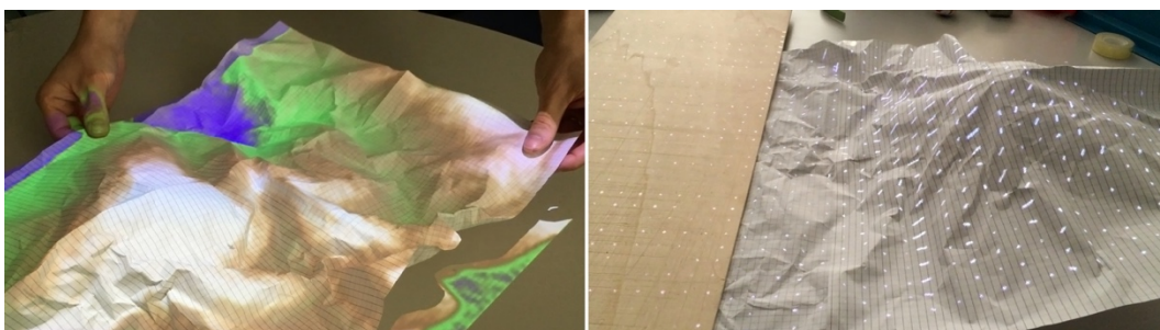
Figure IV-13. Surface analysis in augmented reality. (Left) The height of the surface is represented using a custom color scale, as in the Augmented Reality Sandbox project. (Right) A visualization of the gradient of the surface using a lattice of vectors.
