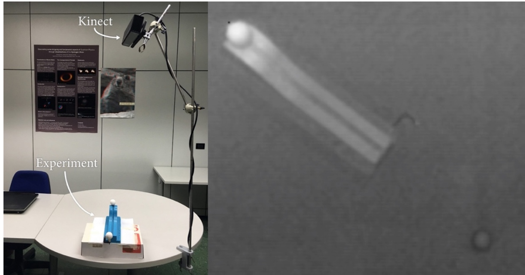
Figure IV-1. (Left) The Kinect is positioned above the environment we would like to reconstruct. (Right) An example of a depth matrix is here visualized as a black and white image, where brighter colors correspond to smaller distances between the sensor and the objects.
