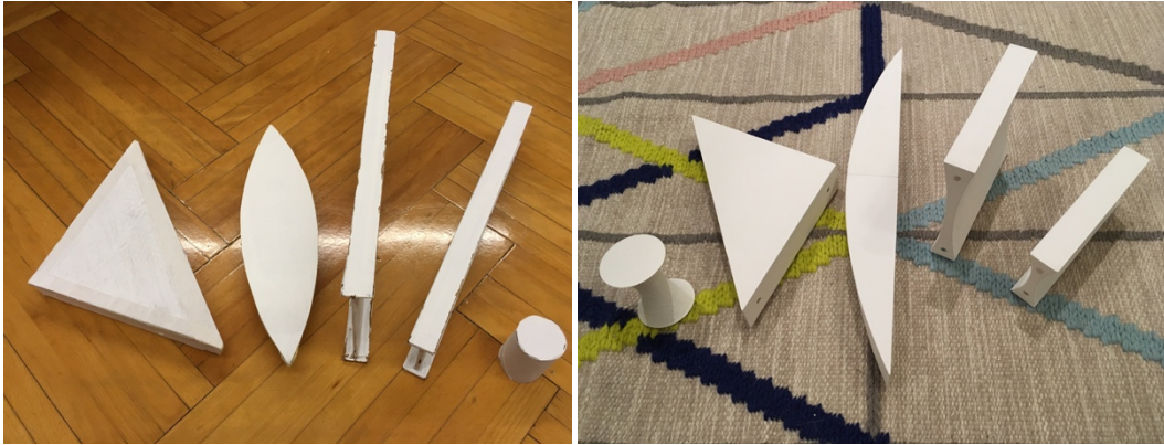
Figure IV-17. Two examples of sets of objects that can be used for the augmented ripple tank. A prism, a lens, a point source, a planar source, and a wall are here represented. (Left) A set made of cardboard. (Right) A 3D-printed set.
