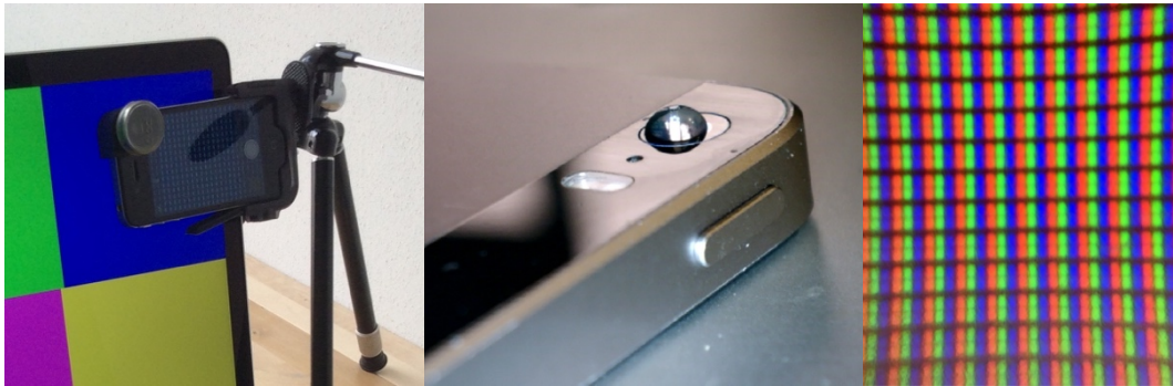
Figure I-34. From left to right: pixels of a monitor seen using an inexpensive macro lens for smartphone; a water droplet on the camera acting as a macro lens; a photo of the pixels taken using the water droplet.
