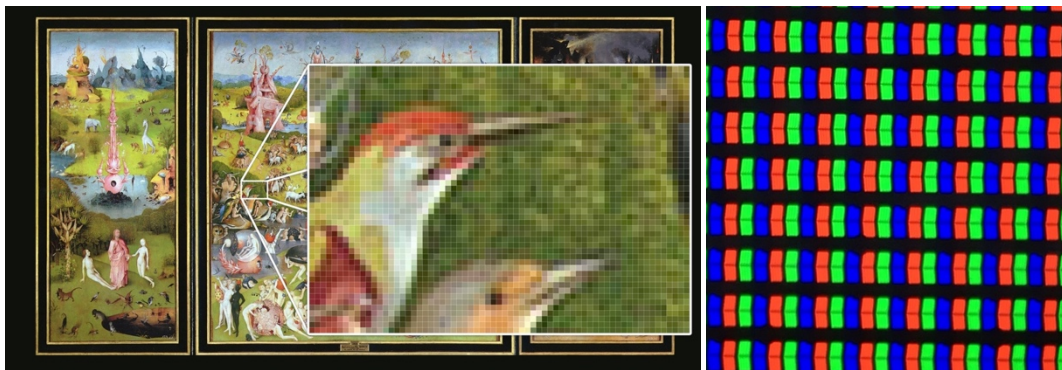
Figure I-7. The pixel of an image, and the pixel of a monitor.
