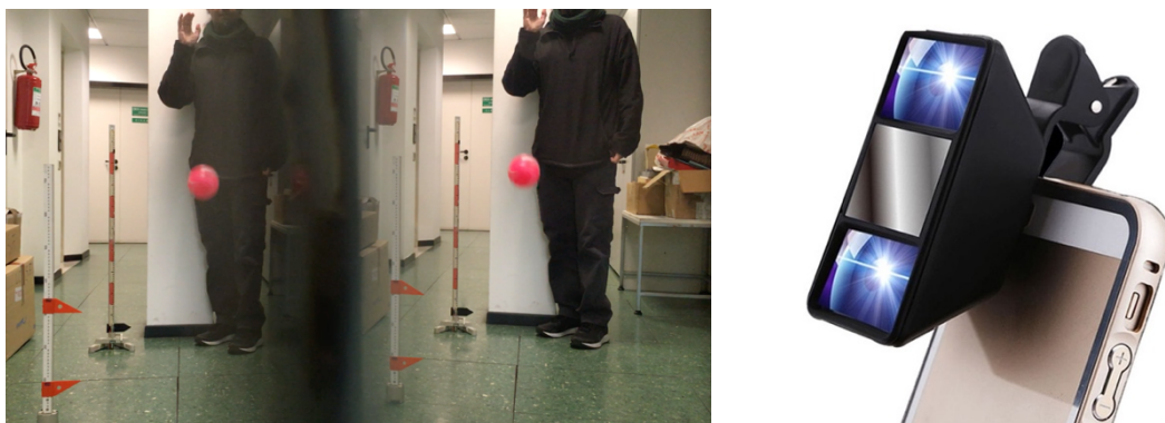
Figure I-39. A screenshot of a stereo video of a bouncing ball taken with a smartphone and a stereo apparatus. The device is depicted on the right.
