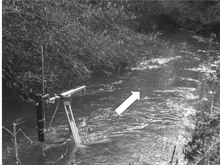
Figure 3.11 Mounting of the Acoustic Doppler Velocimeter formed by a tripod and a metallic mobile frame. The flow direction is represented by the white arrow.
