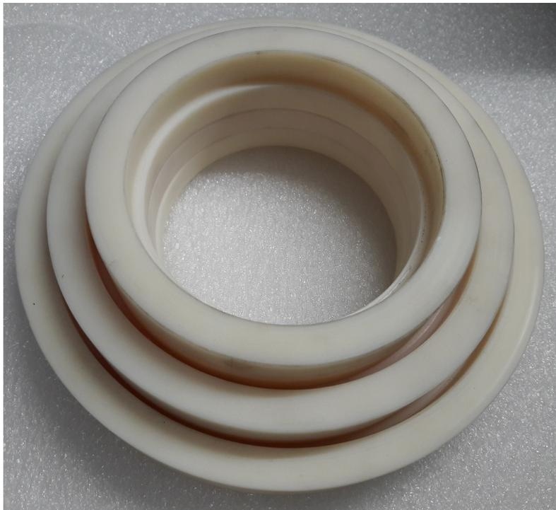
**Figure 5.14:** Set of nylon supports used to correctly arrange the magnetic shield, since they provide the right axial and radial spacing between each next layer.
