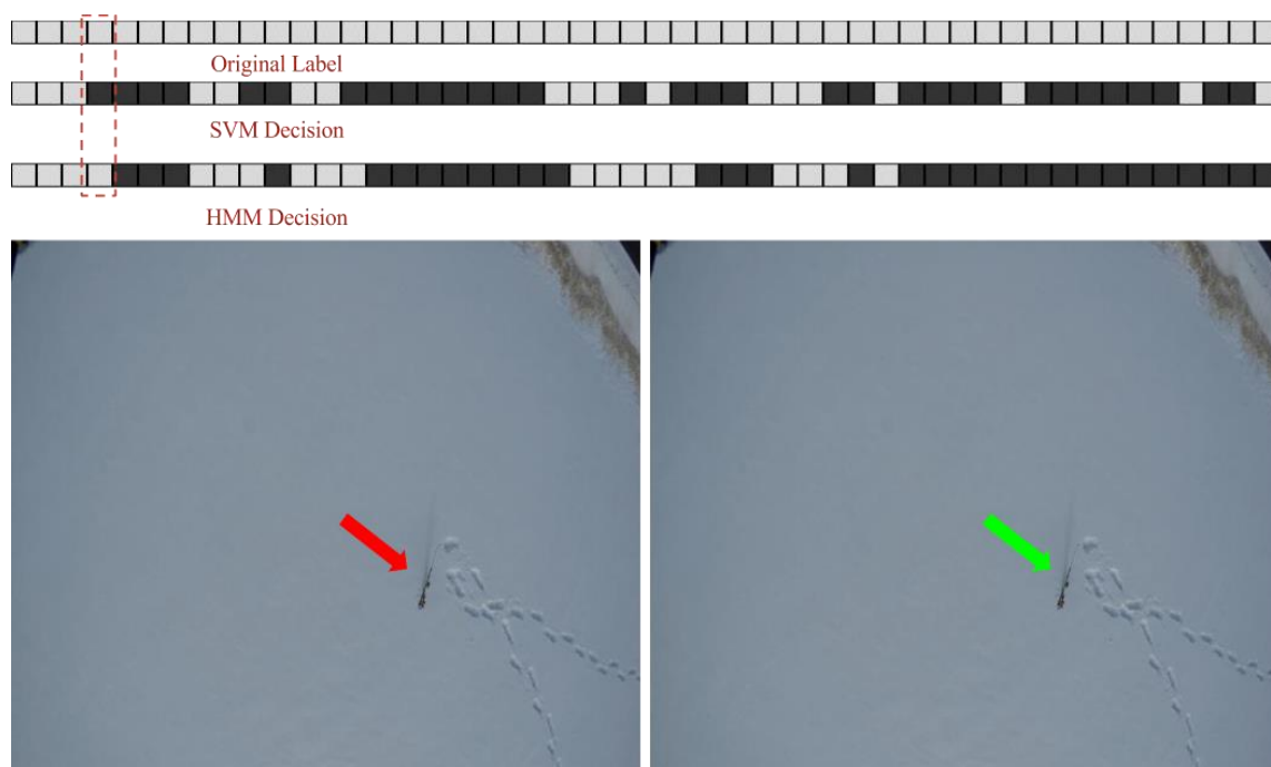
Fig. 2.11. Example of positive change by HMM. Sequence of white and black squares on top indicate label of successive frames. White square indicates a frame has object of interest whereas black square indicates the opposite. The frame where the change happened is highlighted by red dotted rectangle and the corresponding frame in the bottom. The frame for which SVM made wrong decision is shown in bottom left (the object in the frame, skis in this case, is indicated by red arrow) whereas the same frame corrected by HMM is shown in the bottom right (the object in the frame is indicated by green arrow). Note that object is not localized since post-processing decision is made at the frame level.
