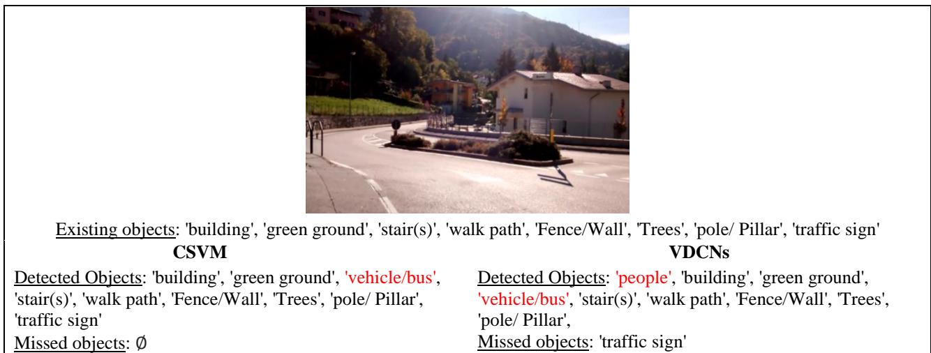
Figure 5-10: Example of classification results with CSVM and VDCNs on Dataset3. In red are highlighted false positives.
