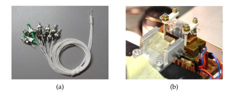
FIGURE 3.8: (a) The picture of fiber array that consists of thirteen 1 meter long fibers. (b) Zoomed view on the optical fiber array positioners and the chip under the PDMS microfluidic flow-cell fasten on the chip holder.
