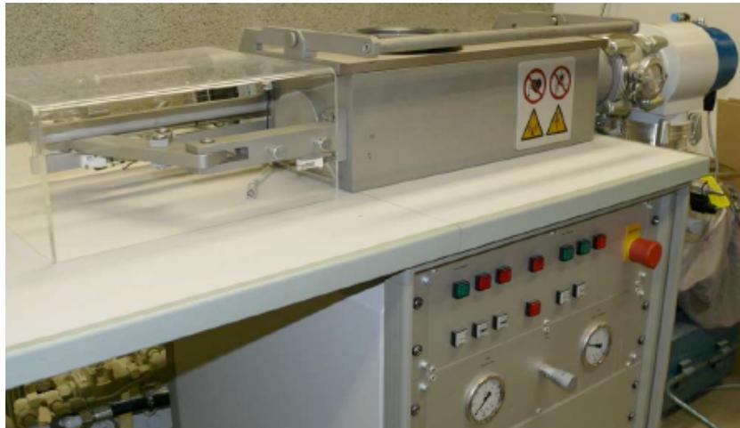
**Fig 24.** Baehr plasto-dilatometer 805 A/D equipped with a compression head
