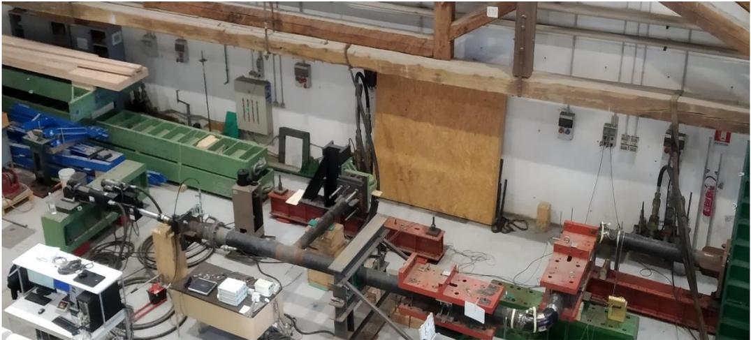
**Figure. 2.19:** Experimental setup, physical substructure of hybrid simulator.
