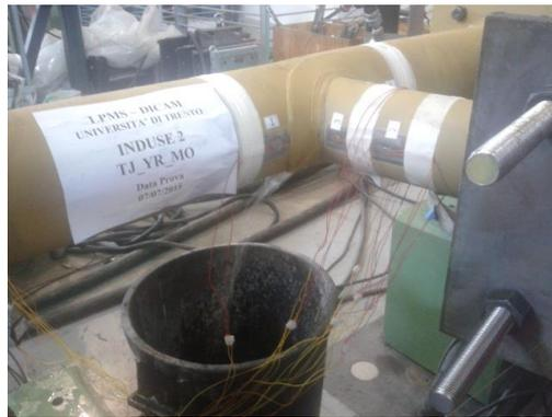
**Figure. 2.14:** Leakage detection during the test of the reinforced specimen under monotonic loading.
