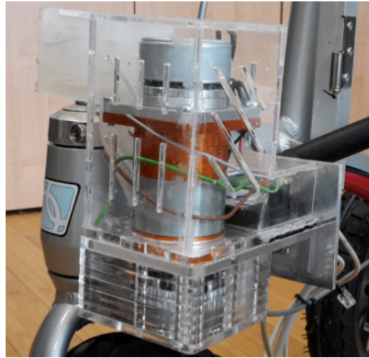
Figure 3.4: Motor mounted on the front right wheel inside the corresponding carter.
