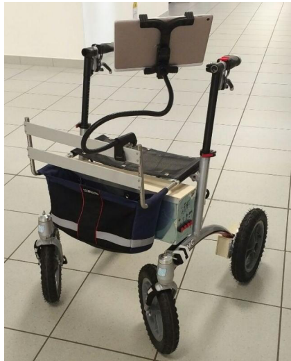
Figure 1.7: FriWalk prototype equipped with the tablet interface [8].
