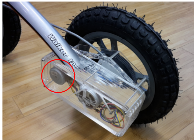
Figure 3.3: Rear wheel of the prototype. The motor is encircled in red.
