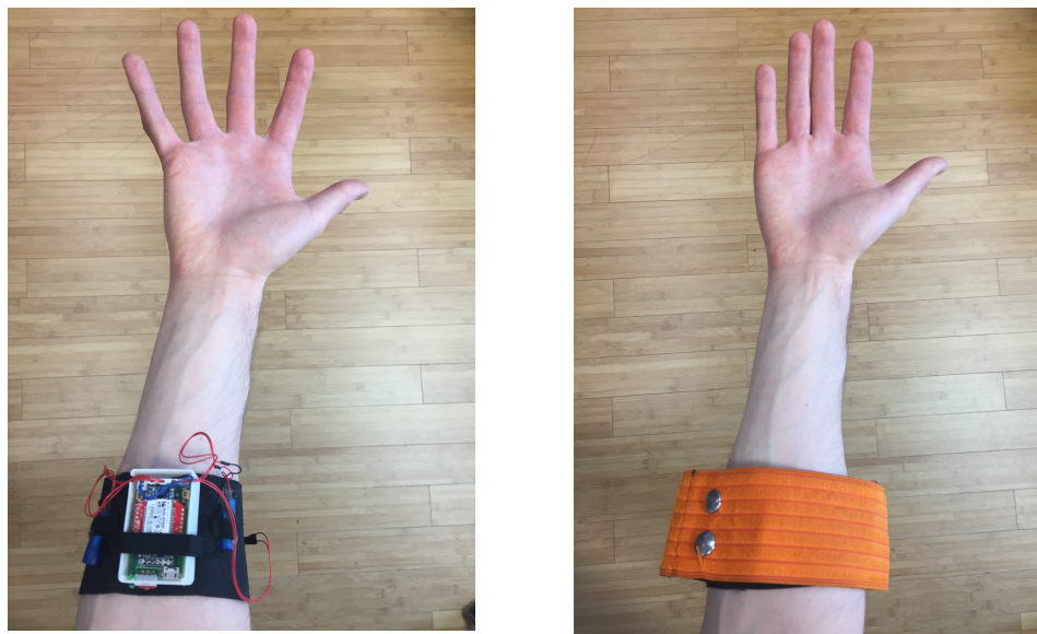
Figure 3.6: Picture of the vibrating bracelets. Placement of vibro motors and board (on the left), device available to the user (on the right) [8].
