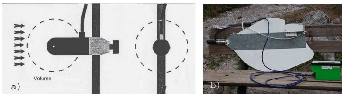
Figure 5.12.: Flux meter: a) scheme; b) device with logger and rudder.
