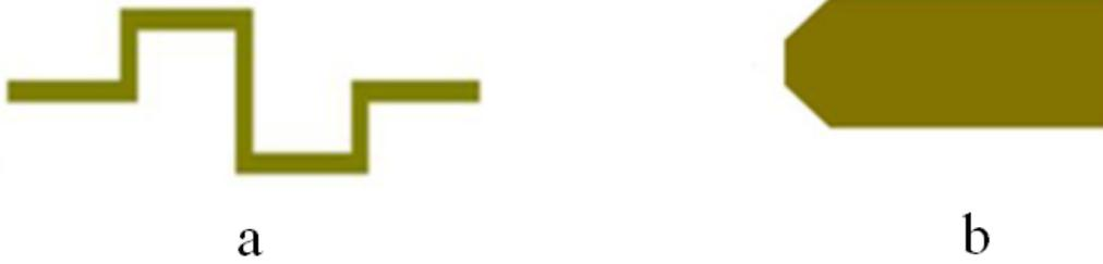
Figure 6.30: Detailed view of the a ) meander spring and b) leaf type spring in thin gold.
