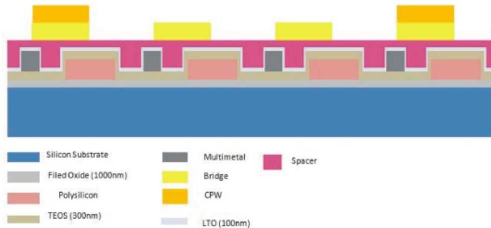
Figure 6.1: shows the cross section of the general design.
