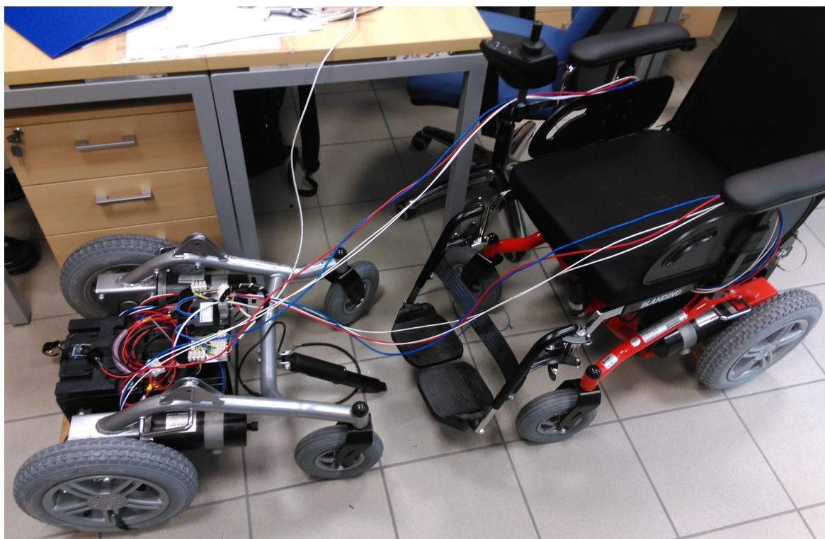
Fig. 5.12 Testbed for the calibration of the wheelchair kinematic parameters.
