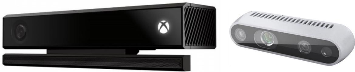
Fig. 5.10 3D cameras: Kinect v2 on the left vs Intel RealSense D435 on the right.
