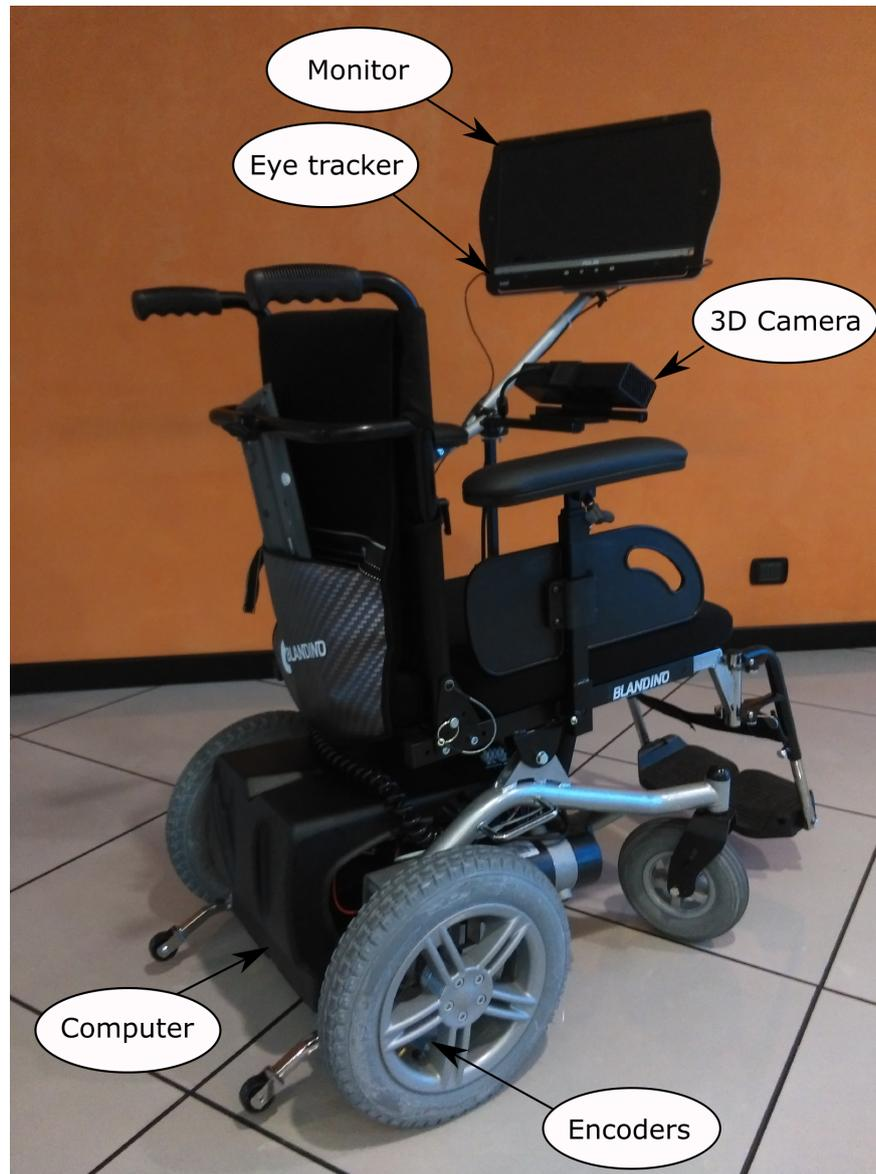
Fig. 5.6 Prototype of semi-robotic eye controlled wheelchair.
