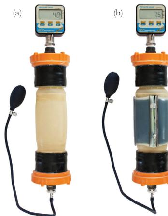
FIGURE 3.3: Testing of the prototype dynamic bandages: air chamber that mimicked the compliance of a human limb, without (a) and with (b) the bandage.
