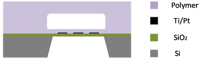
Fig. 1B. Cross section of the TMAH wet etched silicon membrane
