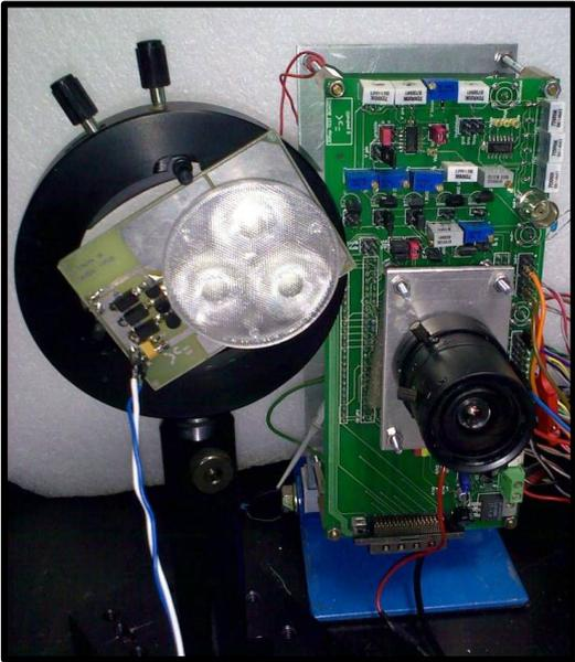
Fig.6.15: Micro Photograph of 3D imager With illumination module
