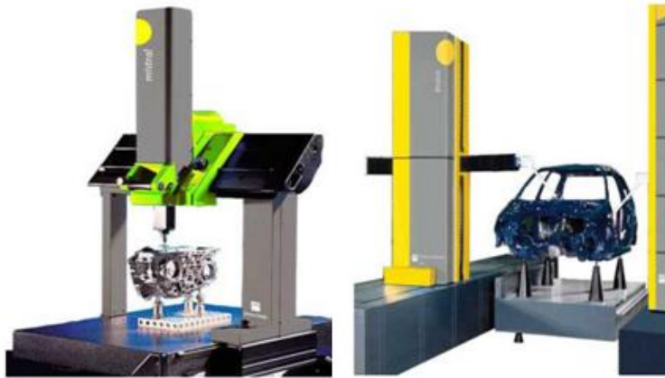
Figure 3.3: Example of contact based system
