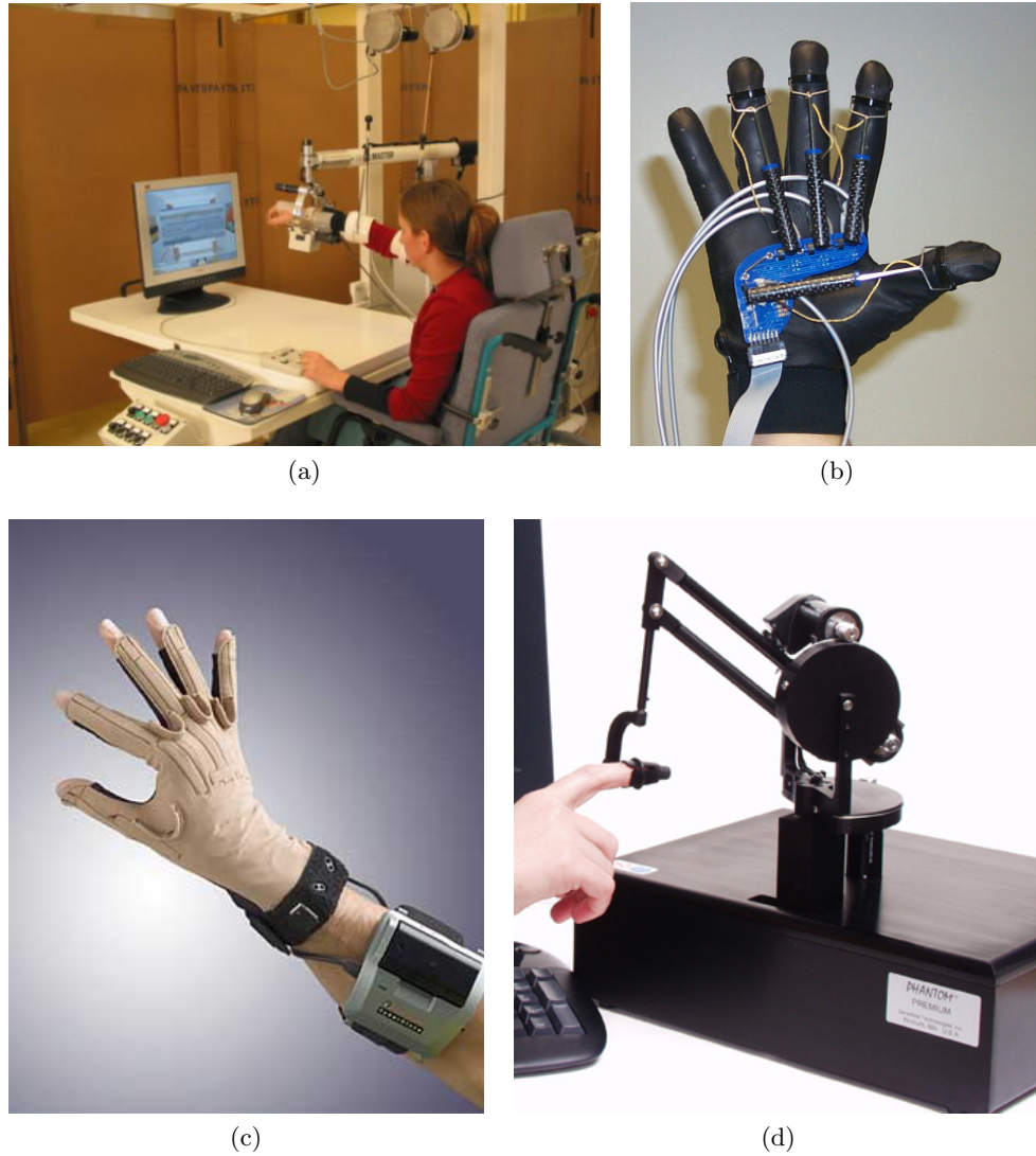
Figure 1.2: Other robotic devices used for rehabilitation: (a) The GENTLE/s device. (b) The Rutgers Master II-ND Glove. (c) The Cyberglove. (d) The PHANTOM device.
