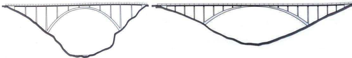
1. 47 High arch: pleasing appearance is created by open spandrel above arch crown Shallow arch: deck and arch are joined at crown.
