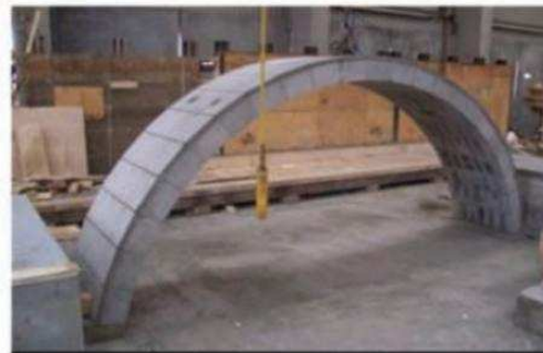
d. Arch positioned on tapered seating units
