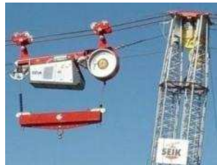
1. Steering pulley block; 2. winch; 3. hoisting rope; 4. crane position; 5. main cable; 6. pulley block; 7. anchorage 4. 29 Hoisting system
