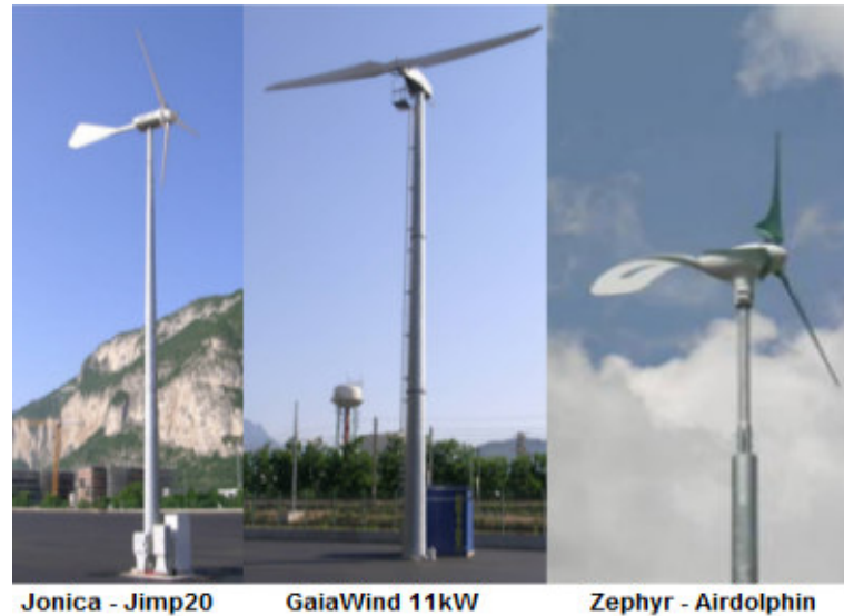
Figure 26: Wind turbines installed at Trento test site
