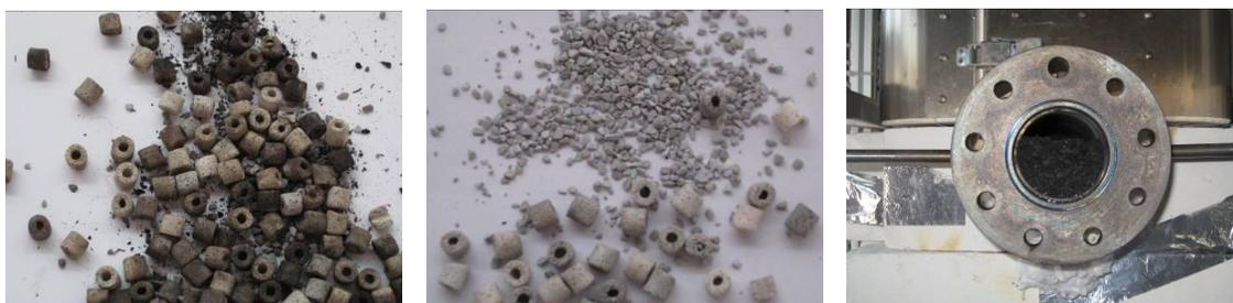
**Figure 3.28** Catalyst after the test at the beginning (left) and at the end of the filter (centre), the connection tube full of char (right)
