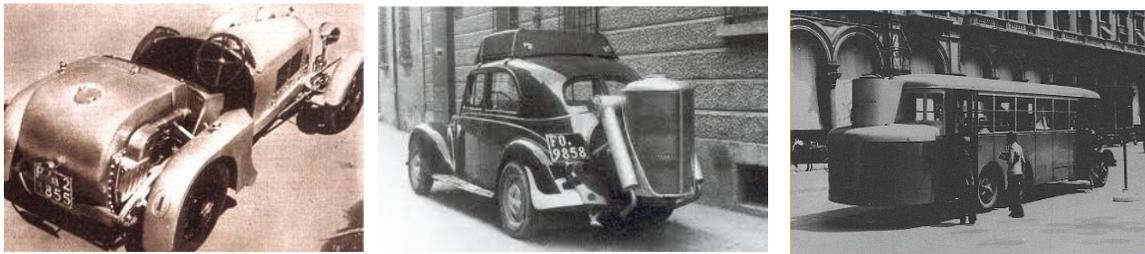
**Figure 1.4** Cars powered by internal combustion engine with wood gasifier. From the left, Alfa Romeo 1750, Fiat 1100 modified by Baldini in 1946, bus used for public transport in Milan during 1930-40s.
