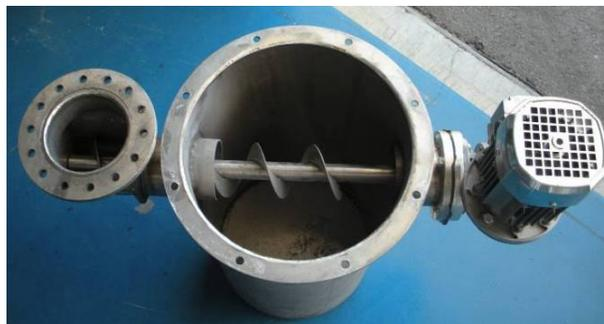
**Figure 3.19** Char collector with the Archimedean screw placed below the reactor
