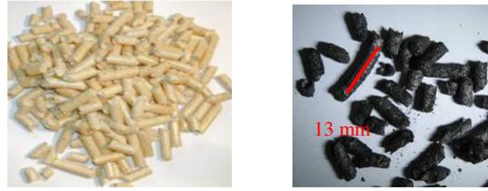
**Figure 3.9** Fresh pellets (left) and gasified pellets (right)
