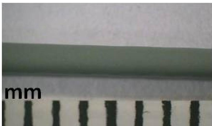
Figure 3.25. Photograph of the anode layer deposited with the slurry at 80 wt% (green state).
