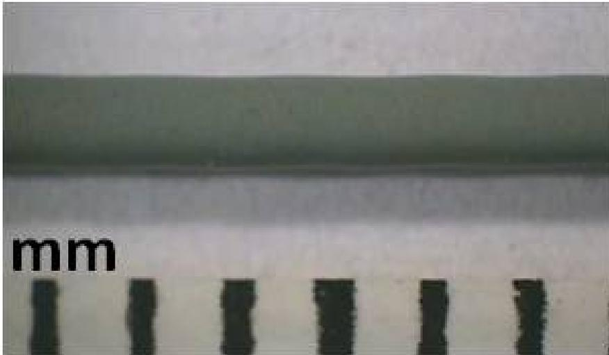
Figure 3.26. Photograph of the anode layer deposited with the slurry at 85 wt% (green state).
