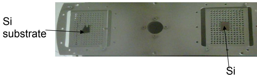
3. Fix the substrate holding plate onto the substrate holder inside the chamber.
