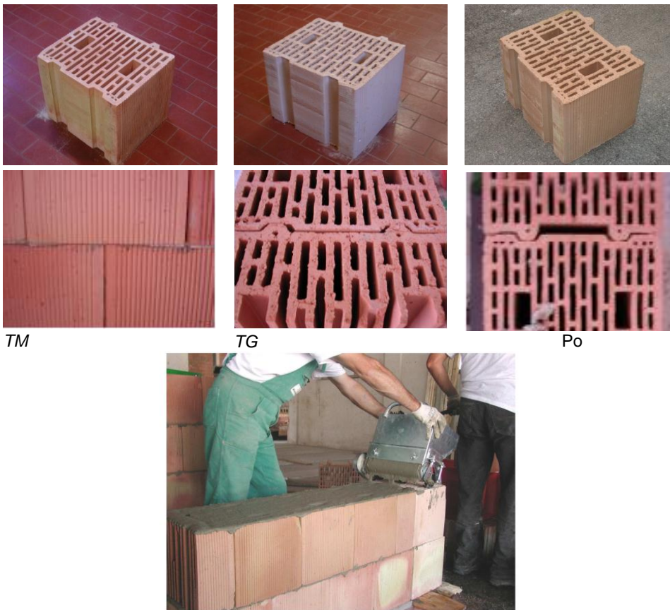
Fig. 3.1. The three masonry unit types respectively: TM TG and Po (above) and construction of a specimen for Thin-layer Masonry (below)
