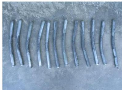
Figure 4.15 (a) Test on specimen with 12 dowels of 16 mm in diameter; (b) Connection failure mode after test (ultimate state for joint); (c) Dowel deformation after test (modified from Polastri *et al.* 2008)
