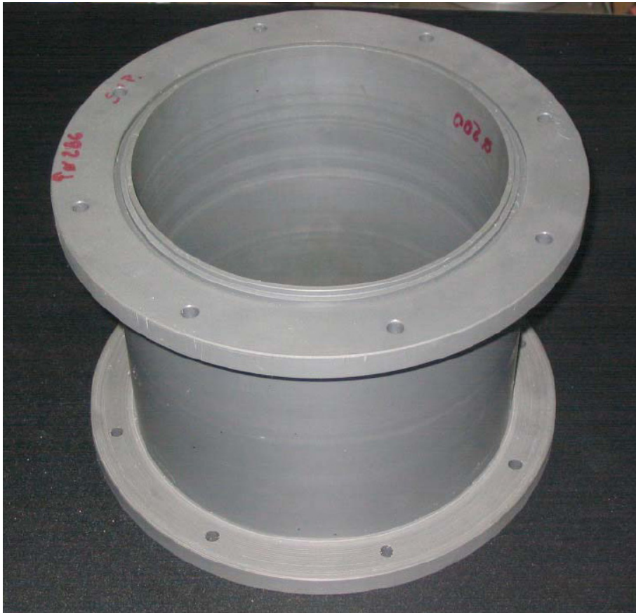
Figure 4.10: Column module in PVC, 20cm high and 20 cm long.
