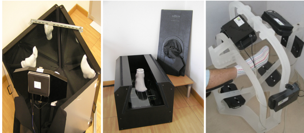
Figure 2.19: The scanner used for the experiment: silhouette (left), laser (centre) and multiple stereo vision (right) technologies.
