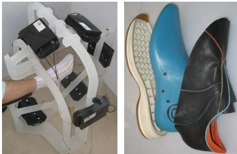
Figure 4.3: The scanner of the foot (left) and the last in-between the sole and the upper (right).
