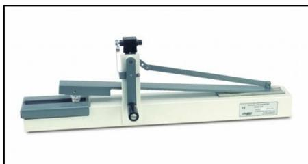
Figure 3.7 *Crockmeter test* [33].
