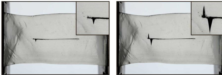
Figure 1.3: Growth of two fractures at the end of an aluminum platelet embedded in a two-component epoxy resin sample (sample S2, see appendix A) under tensile loading (photos taken at the University of Trento, experiment performed by G. Noselli). Both fractures have initiated horizontally (at a mean stress near to 30 MPa), where the stiffener is still attached to the resin.
