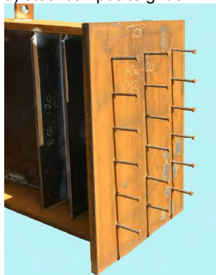
Fig. 11 Examples of Girder End Detail Used in UK (Iles, 2006)
