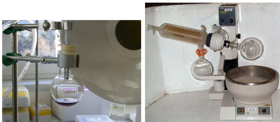
Figure 5.3: Pictures of argon-flow (left) and rotovapor (right) apparatus to coated iron oxide core with dried film.
