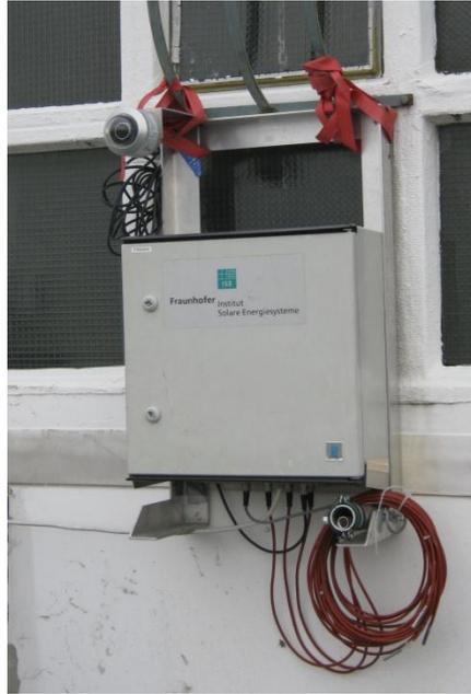
**Figure 5.6** Monitoring of the radiation on vertical surface facing south
