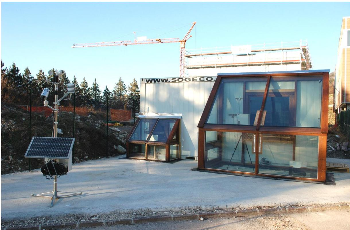
**Figure 4.2** The two sunspaces attached to the container and the measuring instruments
