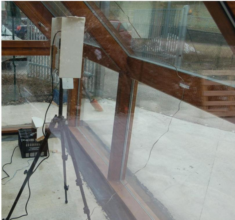
**Figure 4.7** Inside the sunspaces the thermo-hygrometric conditions were measured at two different heights. The sensors were shaded in order to avoid the heating due to the incident solar radiation. Moreover, the air velocity and the surface temperatures of the glazed roof panel, of the floor and of the wall were monitored
