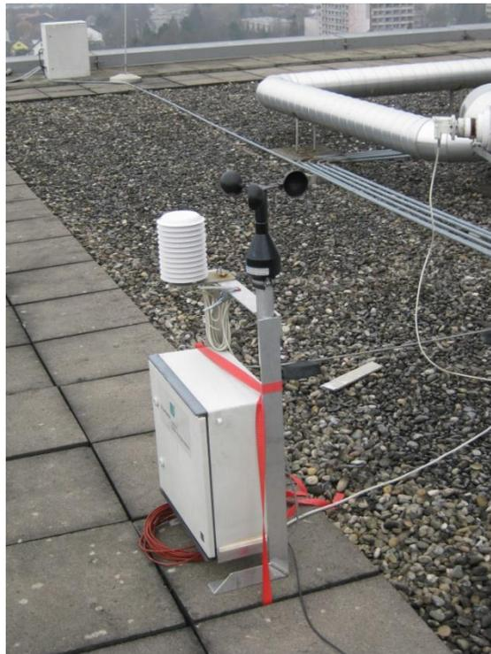
**Figure 5.5** Weather station on the flat roof
