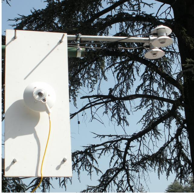
**Figure 2.1:** *Pyranometers used in the experimental test*
