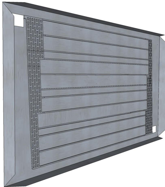
Figure 4.11: Final configurations of the prototype. View on the internal side of the unglazed collector with the channels. The external side is flat. The inlet and outlet pipes are not drawn. Source: Arch. G.Paoletti.
