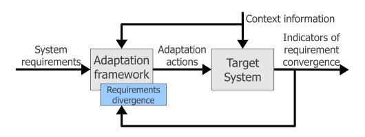
Figure 2.8: View of an adaptive system as a feedback control system.
