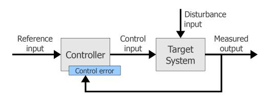
Figure 2.7: Simplified block diagram of a control system based on [Hellerstein et al., 2004].
