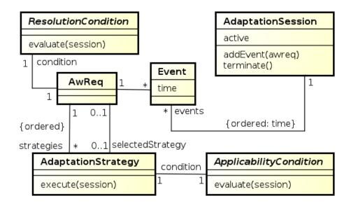
Figure 6.4: Entities involved in the ECA-based adaptation process.
