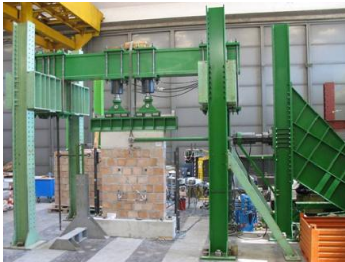
Fig. 3.4 Shear compression test set-up
