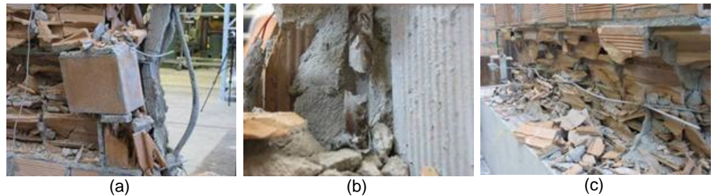
Fig. 3.7 (a) Buckling of vertical bars in TRSa 0.4; (b) tension failure of vertical bars in SRSb 0.4; (c) transverse deformation of truss at end of test in TRHS 0.6.
