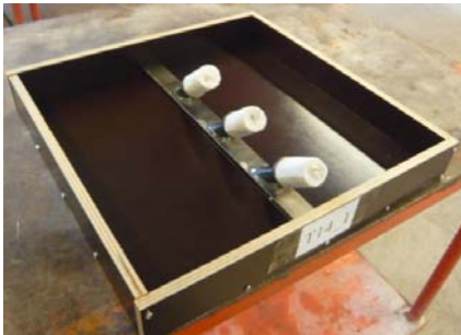
Figure 11: Steel tubes in the formwork before concrete casting
