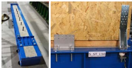
Figure 7: anchor the sill beam and the wall fixings
