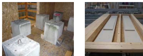
Figure 5: Additional masses on the floors and inside the structural wall
