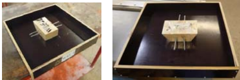
Figure 14: Wooden shear anchor-key before concrete casting. Left: W45-type. Right: W30-type.
