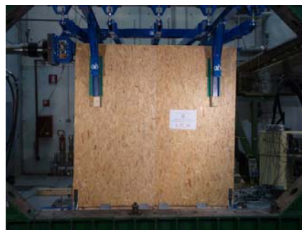
Figure 2: Test Set-up of the tests on framed walls subject to horizontal action (monotonic and cyclic) and different magnitude of vertical load
