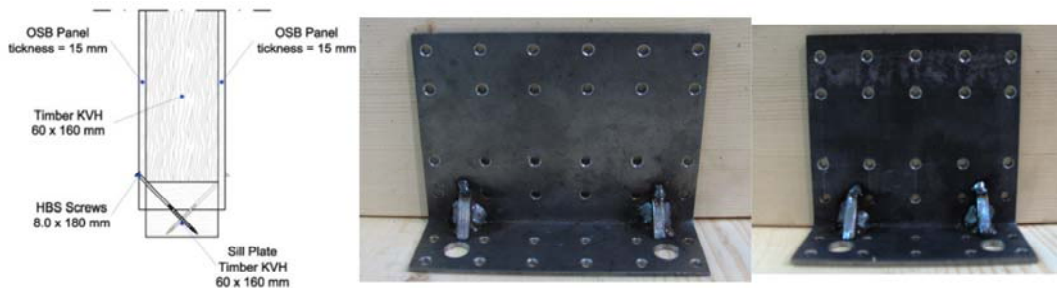
Figure 3- Connection with screws, angle brackets NEW150 and NEW120
