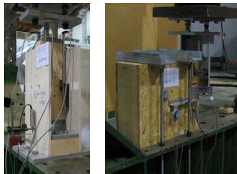
Figure 1: Test Set-up of the tests on the connections between vertical stud and sheathing panel and the connections between wall and foundation
