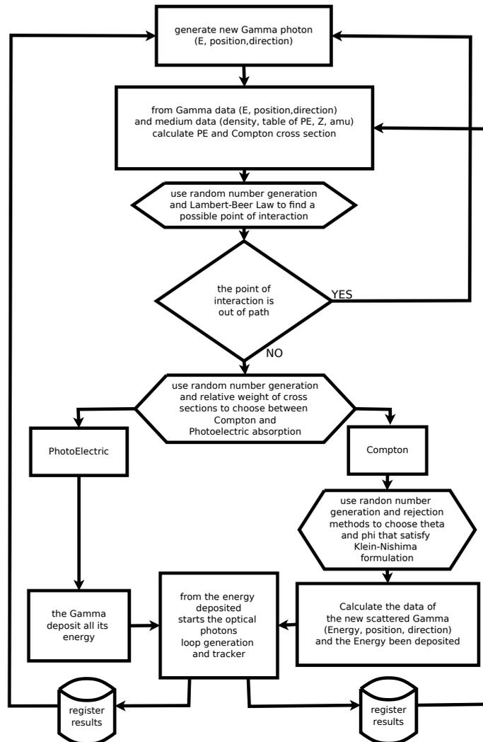
Figure 6.1: Flux diagram of  $\gamma$ -ray generation loop as it is implemented in the SLitrani TGamma class. Being based on the algorithm presented in [90] the flux diagram is pretty similar to the one presented in the original article.
