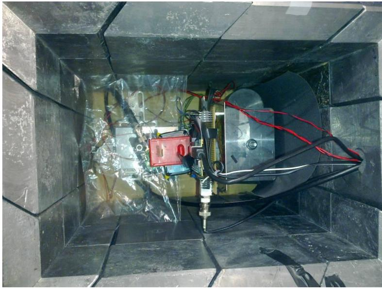
Figure 4.6: Experimental setup used for the experiments with  $\gamma$ -ray sources. It can be noticed the position of the sources that are contained in the red and blue boxes. Two different sources (low activity  $^{133}\text{Ba}$  and  $^{22}\text{Na}$ ) have been used to reach a number of events well discernable from the background radiation activity. The sources are positioned as close as possible to the crystal.
