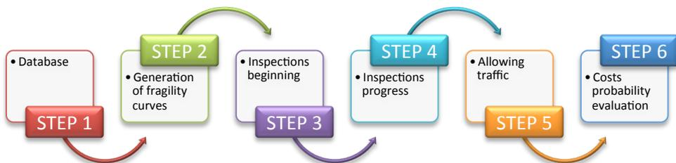
Fig. 3.1 The framework proposed in this study to assess seismic vulnerability of existing bridges after an earthquake mainshock.
