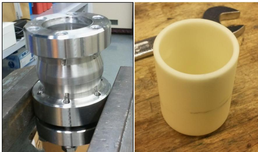
**Figure 6.1** – Metallic containment and ceramic inlay manufactured in alumina ( $\text{Al}_2\text{O}_3$ ).
