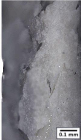
**Figure 33** – Micrograph of SPNCs matrix debonding after the consolidation.
