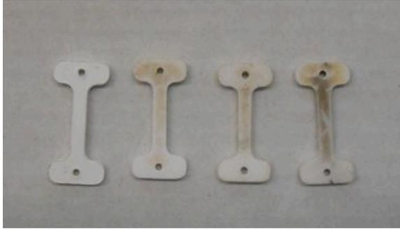
**Figure 5.19 Blackening observed after flash treatment at 800C. Sample grain size increases from left ( $G=0.60 \mu\text{m}$ ) to right ( $G=11.47 \mu\text{m}$ ). The cathodic reaction occurred at the under hole.**
