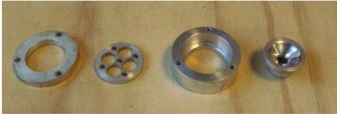
**Figure 4.3: Die setup used for high shear mixing of 8YSZ paste before extrusion [81]**
