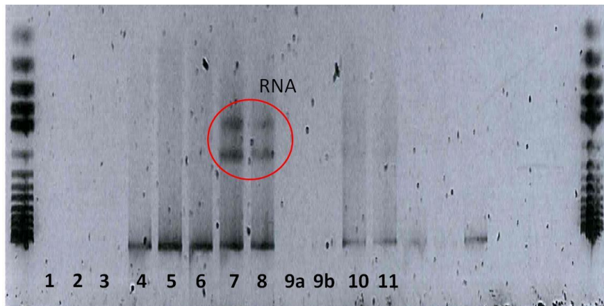
Figure A6 Gel electrophoresis from DNA extract from the same sample with different methods.
