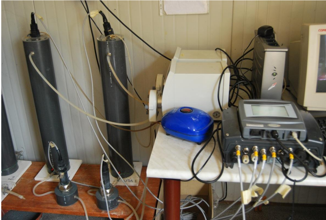
Figure 15 View of the cores under respirometric test.
